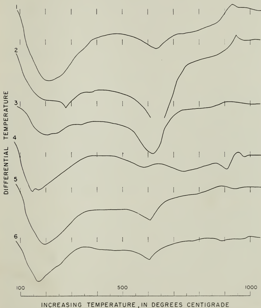
FIGURE 59.—Representative differential thermal curves of soil clays. (Thermal curve numbers correspond to soil clay numbers on facing page.)
