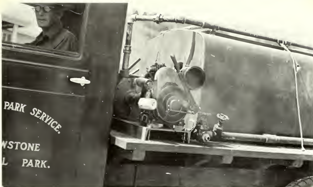
Briggs-Stratton Pumping Unit which provides circulation for the fish tank, - 2-cycle motor.
