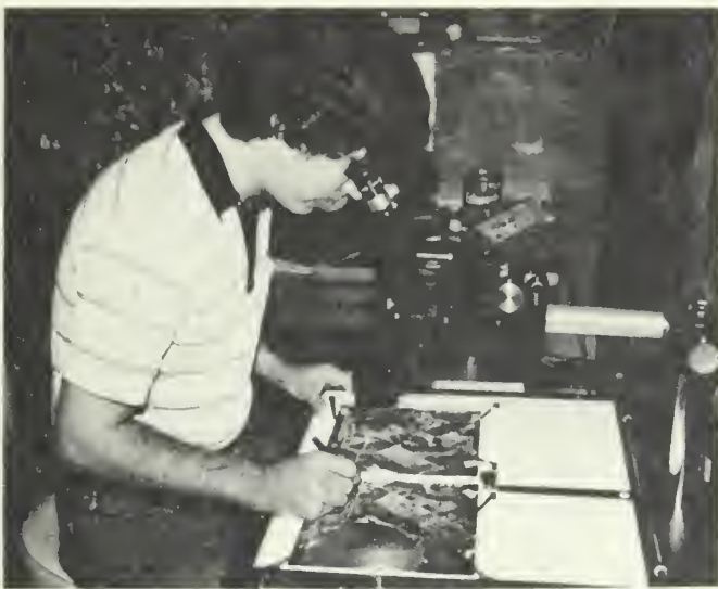
Figure 1(a) —Project forester Charles Bryant delineates forest stands on color infrared stereo aerial photographs, one step in the process of developing southern pine beetle hazard maps. (All photos courtesy Texas Forest Service.)
