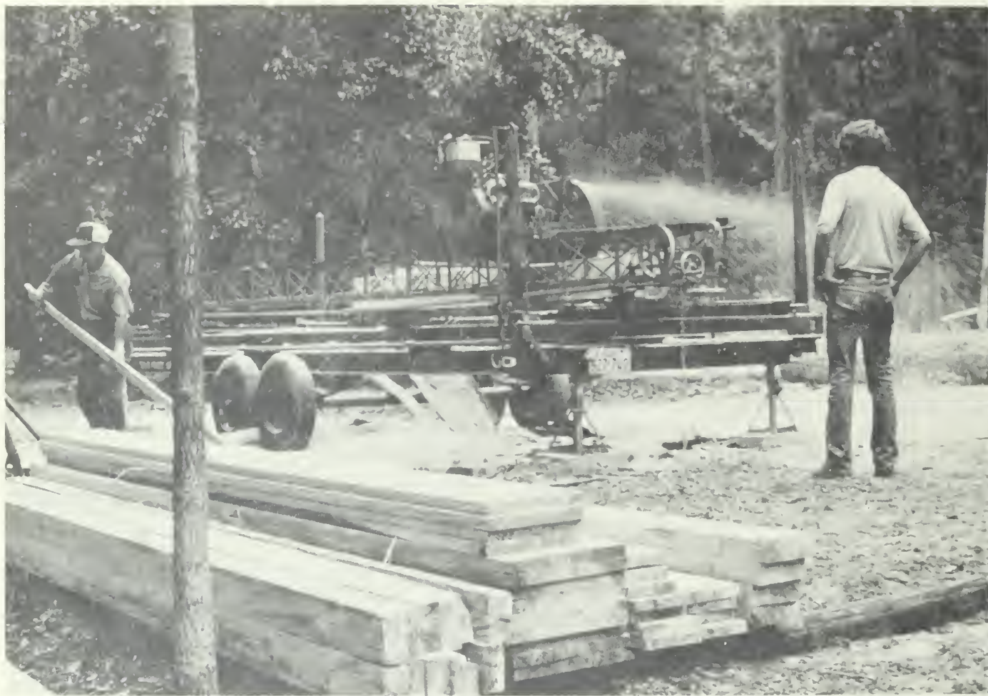
Figure 4(a) —Portable sawmill used in the East Texas Demonstration Project to produce rough-cut dimension lumber from beetle-killed pines.
