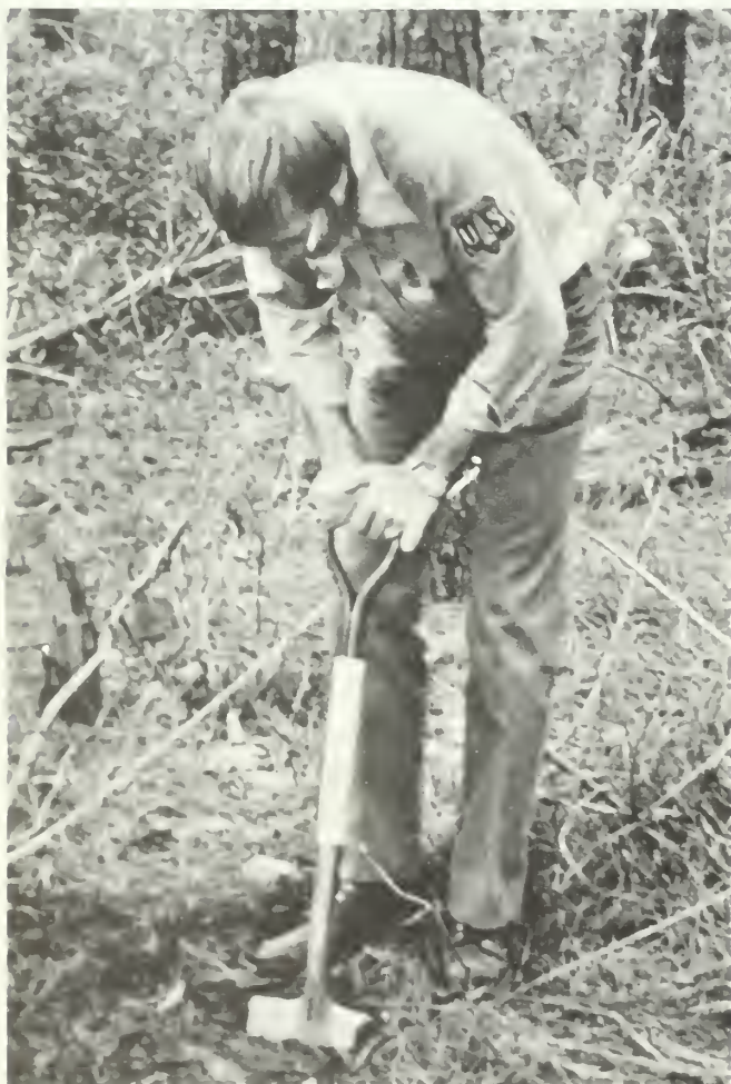
Figure 3 —Removal of cubic-foot soil sample to determine percentage infection of pine roots by annosus root rot.
