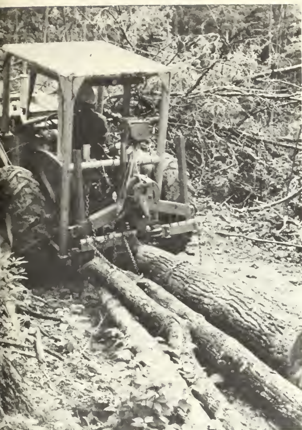
Figure 5.—Farm tractor with rear winch used for skidding residue.
