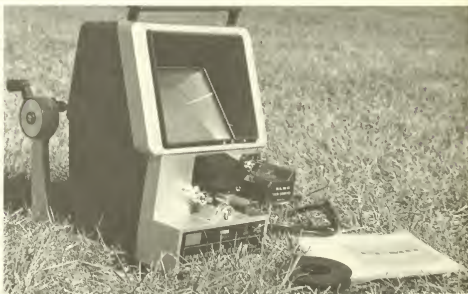
Figure 6.—Editing machine for 8-mm movie film is used to view and analyze film taken by the automatic monitoring camera.
