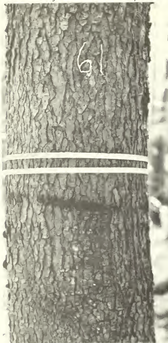
Figure 1.—Paired dendrometers were installed at 4.5 feet above ground on 33 black cherry trees.
