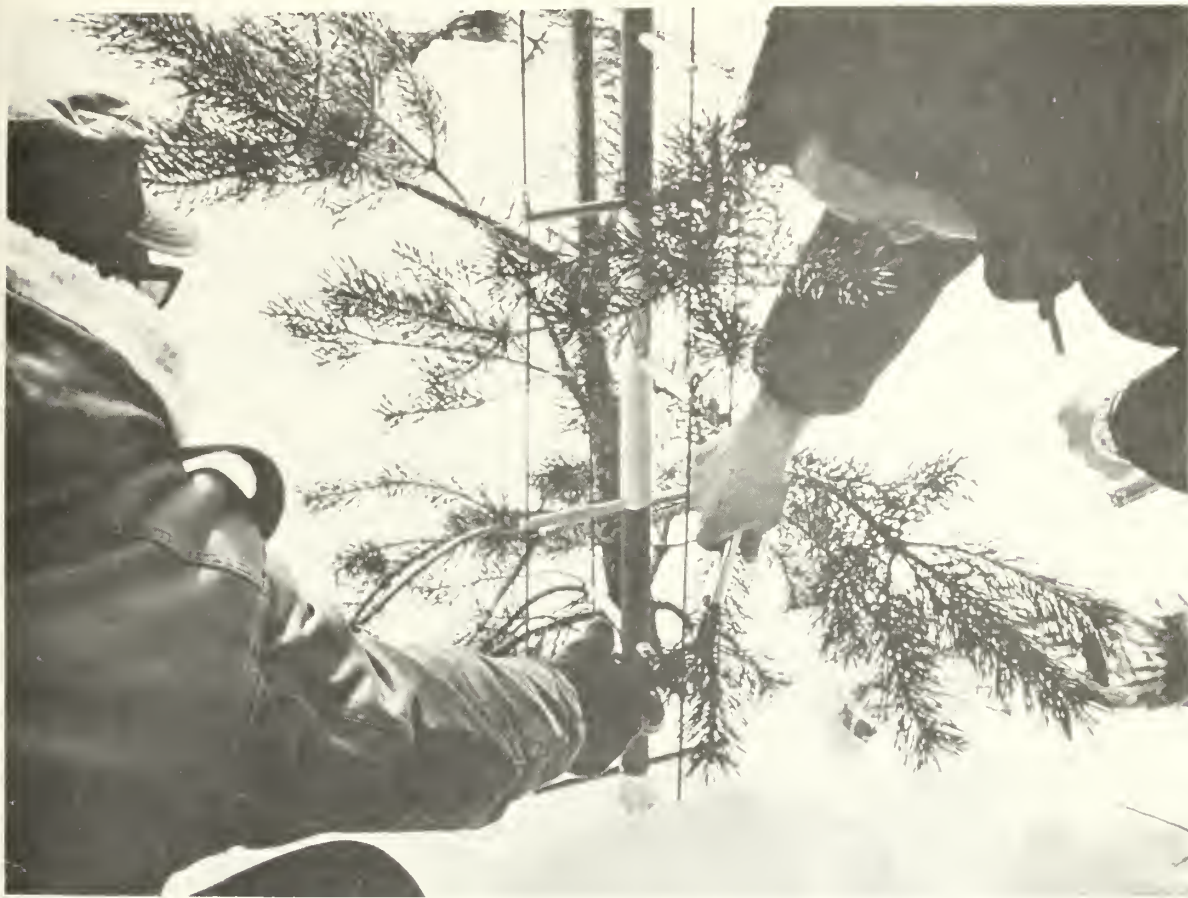
Figure 2.—Detailed view of the sampling pole in use. Sighting wires are being used to locate position for clipping a branch with a hand pruning tool.
