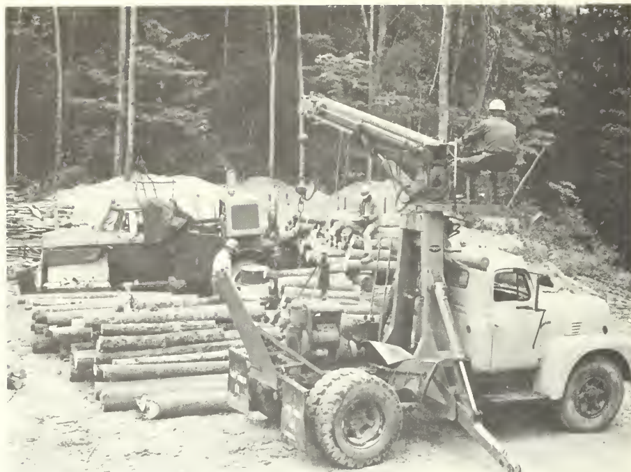
Figure 3.—Weighing and decking sawable bolts from residual trees.
