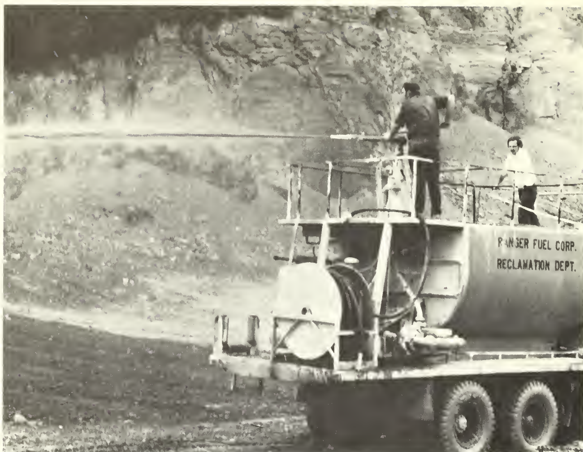
Figure 1.—Hydroseeder applying seed, fertilizer, and bark fines.
