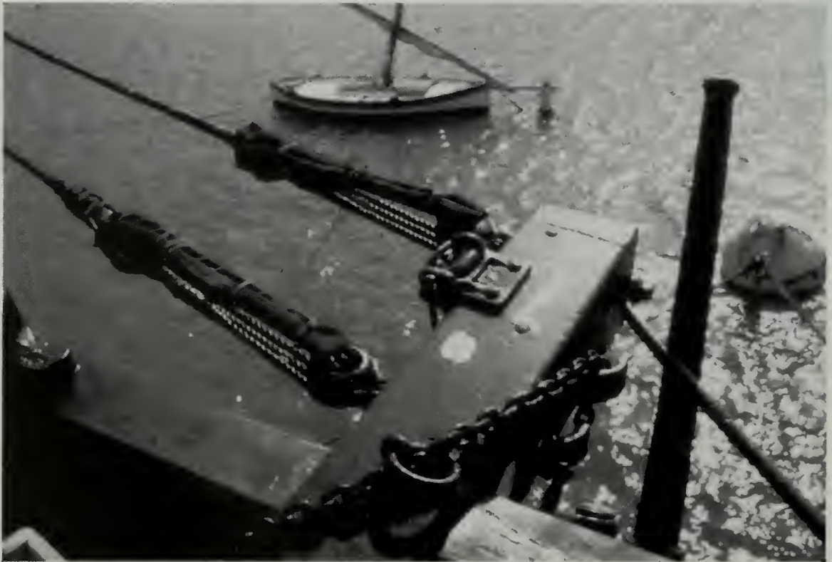
Figure 4.28. Rigging element supporting jibboom guys on forward side of C.A. Thayer's cathead. NPS photo by Matt Russell.
