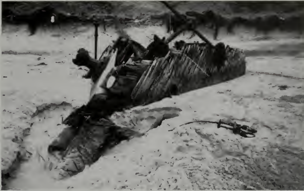
Figure 4.12. Comet's bow. The hawse timbers are in the center with the white float on them. The hawse pipe is visible at the sand-line, to the right of the hawse timbers. In the right foreground is an unattached rigging element. NPS photo by Matt Russell.
