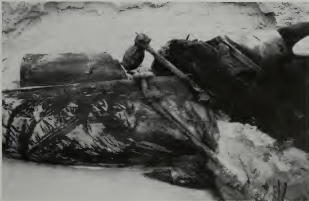
Figure 4.13. Side view of Comet's port knighthead (to the right) and bowsprit where it exits the hull. The jibboom heel chock is on top of the bowsprit. Also visible is the gammon iron and the bull's eye for the fore-stay. NPS photo by Matt Russell.
