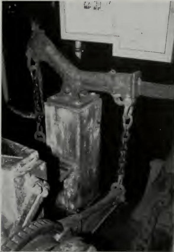
Figure 4.37. Pivoting rocker, or crosshead, mechanism connected to a windlass purchase arm with chain. Comet was equipped with a similar windlass type. NPS photo by Matt Russell.
