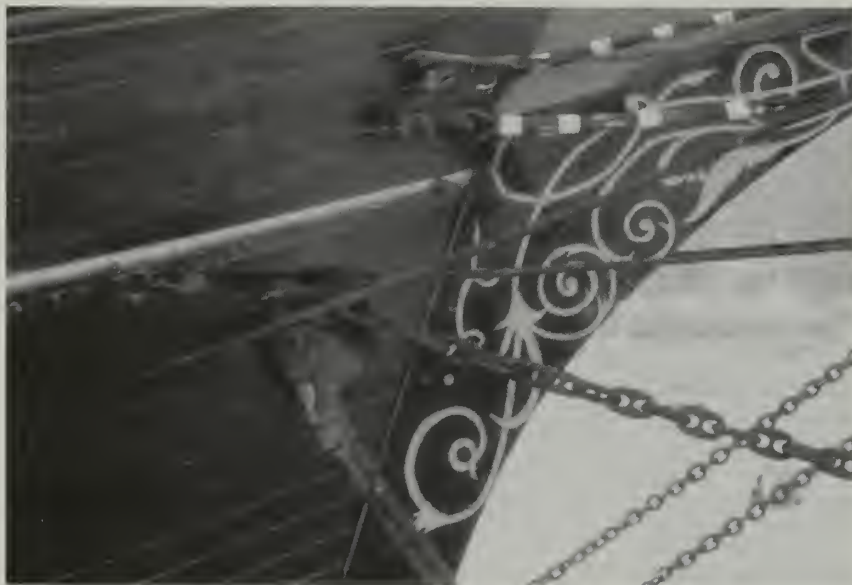
Figure 4.24. Bull's eye above and forward of the hawse pipe (at the top-center of photo) support the bowsprit guys on C.A. Thayer in San Francisco Maritime National Historical Park. NPS photo by Matt Russell.
