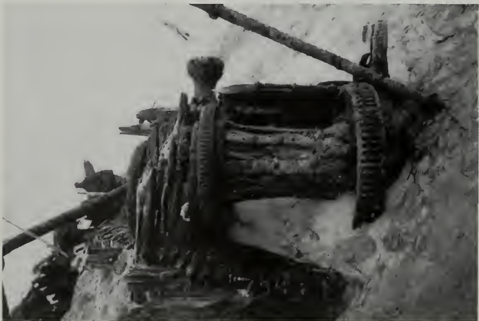
Figure 4.18. Photograph taken from the perspective as if the viewer were standing on the main deck looking forward. The pawl post is to the left of the windlass. NPS photo by Matt Russell.
