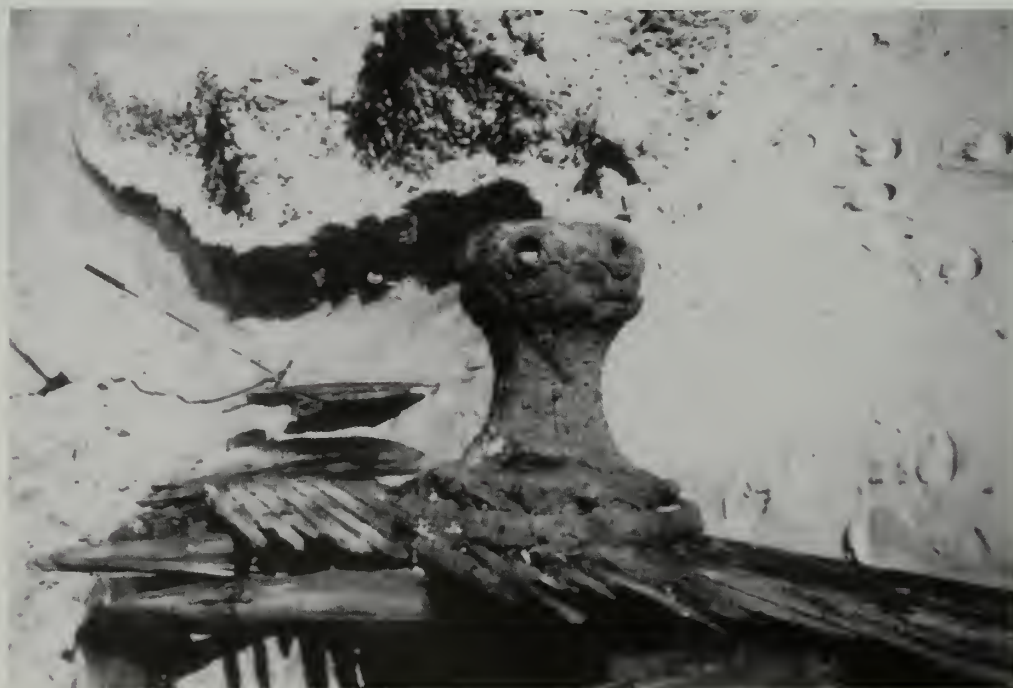
Figure 4.44. Comet ’s capstan, mounted in the center of the forecastle deck. NPS photo by Don Morris.
