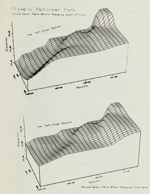
FIGURE 4. THREE DIMENSIONAL PLOT DEPICTING THE GROUND WATER TABLE BEFORE AND AFTER CHANGING THE POND LEVEL
