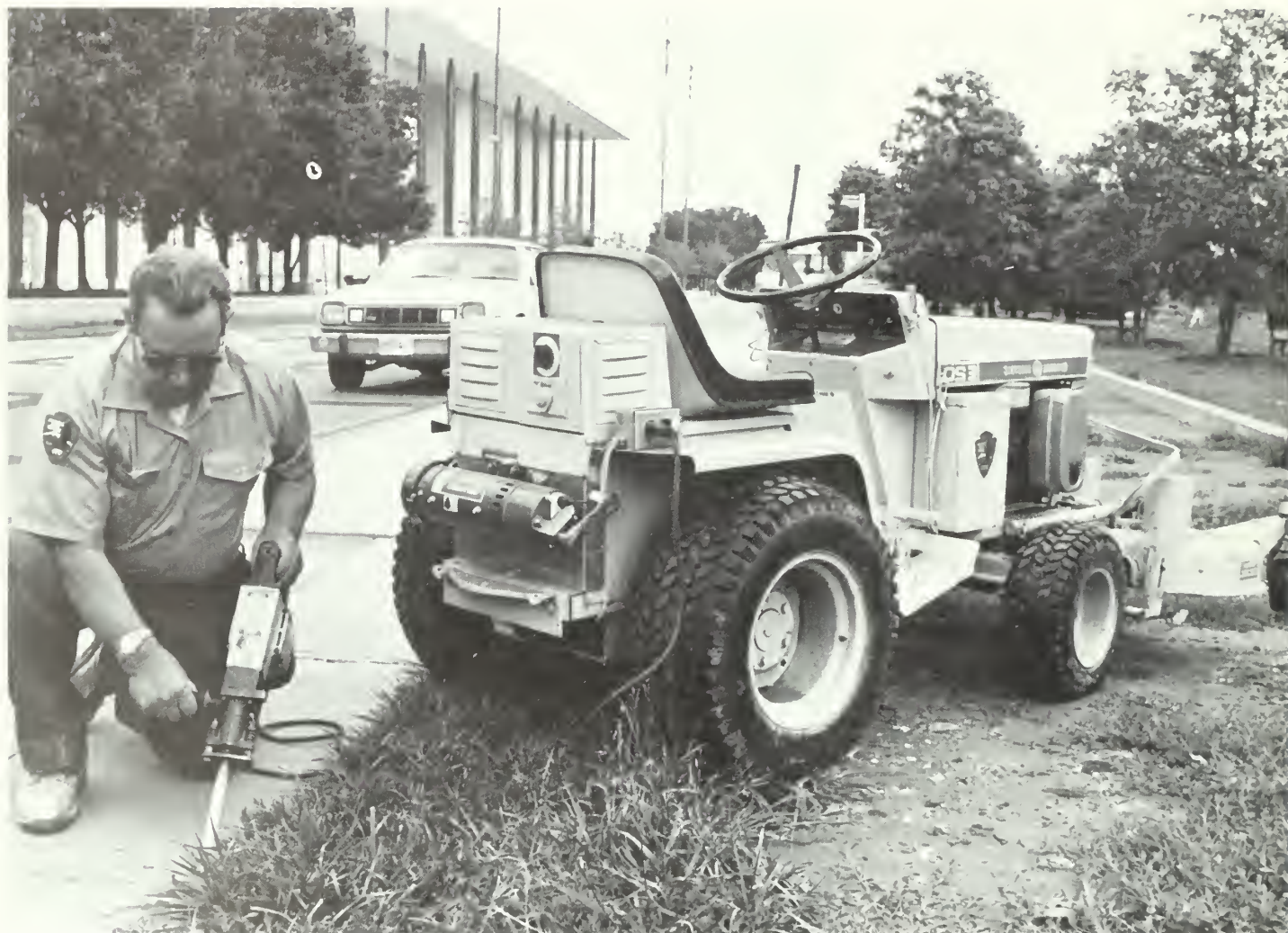
An early-model electric battery-operated tractor can silently operate on a 36-volt battery pack.
