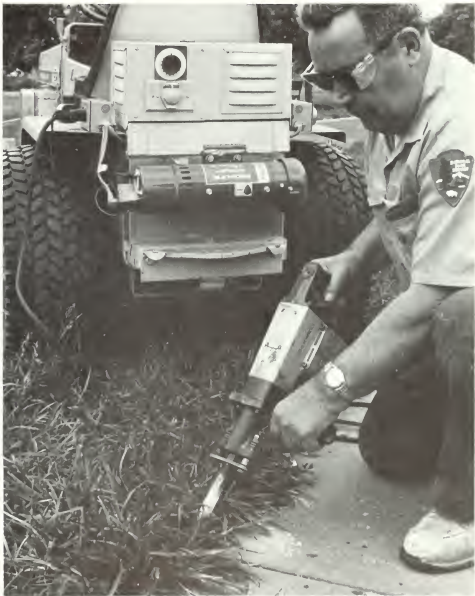
An AC power tool is plugged into the fender-mounted AC outlet of this electric battery-operated tractor.
