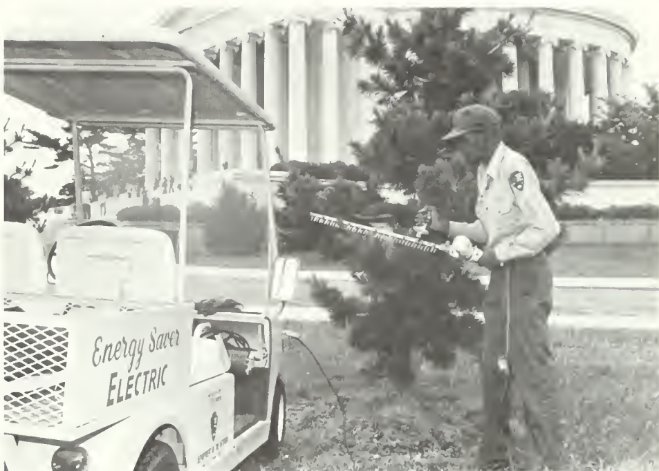
This Site Supervisor electric utility cart is of "footprint" weight on the ground; turf damage is almost nil.
