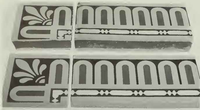
Figure 25. This comparison of an original, historic encaustic tile (top) with a reproduction encaustic tile (bottom) reveals an obvious difference in thickness, but only a slight difference in the design. Photo: Wayne Firth, Office of the Architect of the Capitol.
