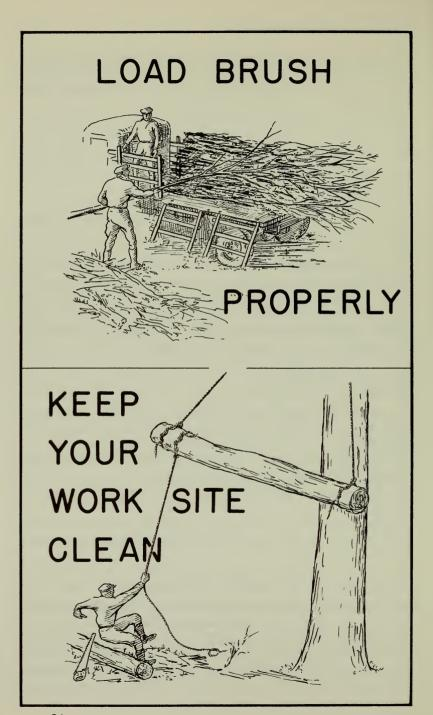
to cars passing around the truck and prevents the brush from scraping cars or striking pedestrians. Whenever brush extends beyond the confines of the truck, red flags should be placed on the ends. (See page 24.)
