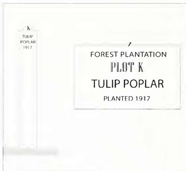
Figure 5: Suggested design for post (boundary) and signboards to identify the forest plantations. Signs should be attached with fasteners that do not damage trees. Not to scale. (SUNY ESF.)
